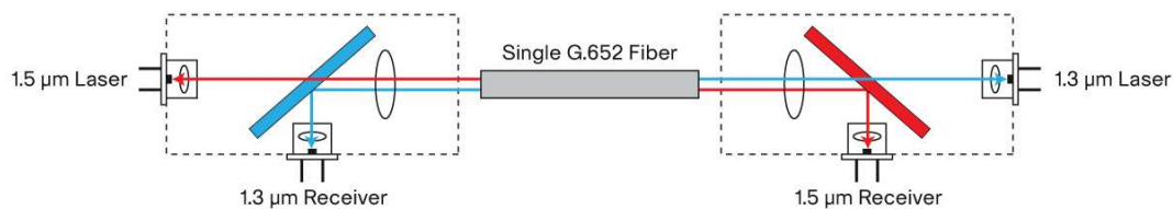
Figure 2. Bidirectional Transmission on a Single Strand of SMF
